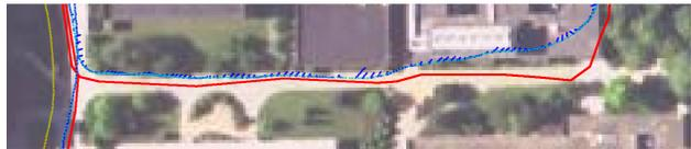
**Figure 8.** Close up plot of Localization methods vs GPS. Red - Ground Truth. Blue - NavSatTransform. Cyan - Sensor Fusion. Yellow - LOAM.
