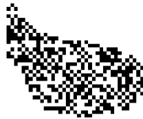
Figure 3. Examples of connected components rendered with a halftone pattern. We can see a lot of interleaved pixels in these connected components after binarization, and they cannot be identified by the size limits.
