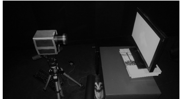
Figure 3. First experimental setup. The illuminance meter is set 0.60 m away from the monitor, and focuses on the displayed image patch let through by the cardboard mask. Images within the image set were displayed in an orderly fashion, from biggest to smallest minimum luminance squares. All lights were switched off for the whole duration of the experiment.
