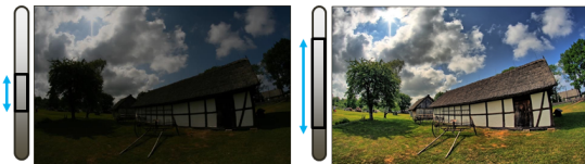
Figure 1: LDR and HDR images. (left) LDR image (right) HDR image, peak luminance and colorfulness of HDR image are higher than LDR image.
