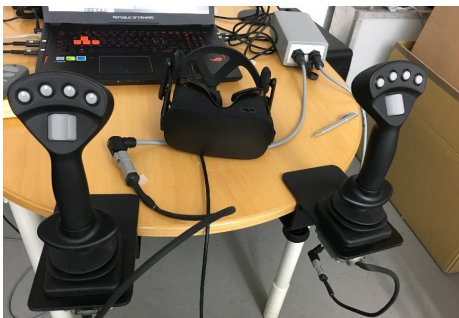
Figure 2: The two joysticks for operating the crane in the VR simulator and the HMD of the brand Oculus Rift
