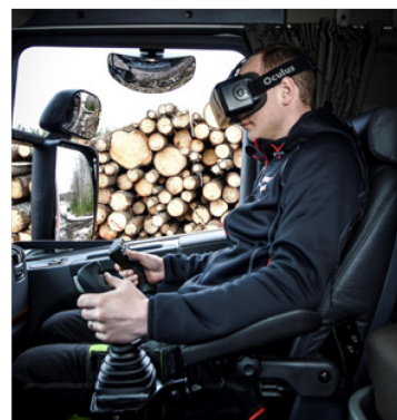
Figure 1: Photo of VR-goggle based crane operation from inside the Truck cabin
