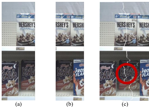
Figure 4: Photoshop stitching. (a) Left and (b) right images lack a featureless area, forcing the stitching seam to pass through highly structured areas located at depths different than the optimal depth. (c) Stitched image shows duplicated content (circled) in the back objects.
