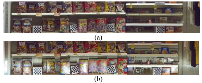
Figure 11: Stitching comparison with different lighting. (a) The stitched image with normal room lighting has darker areas (right) that are more challenging for depth estimation. (b) The stitched image with an additional light source attached to the camera performs better.
