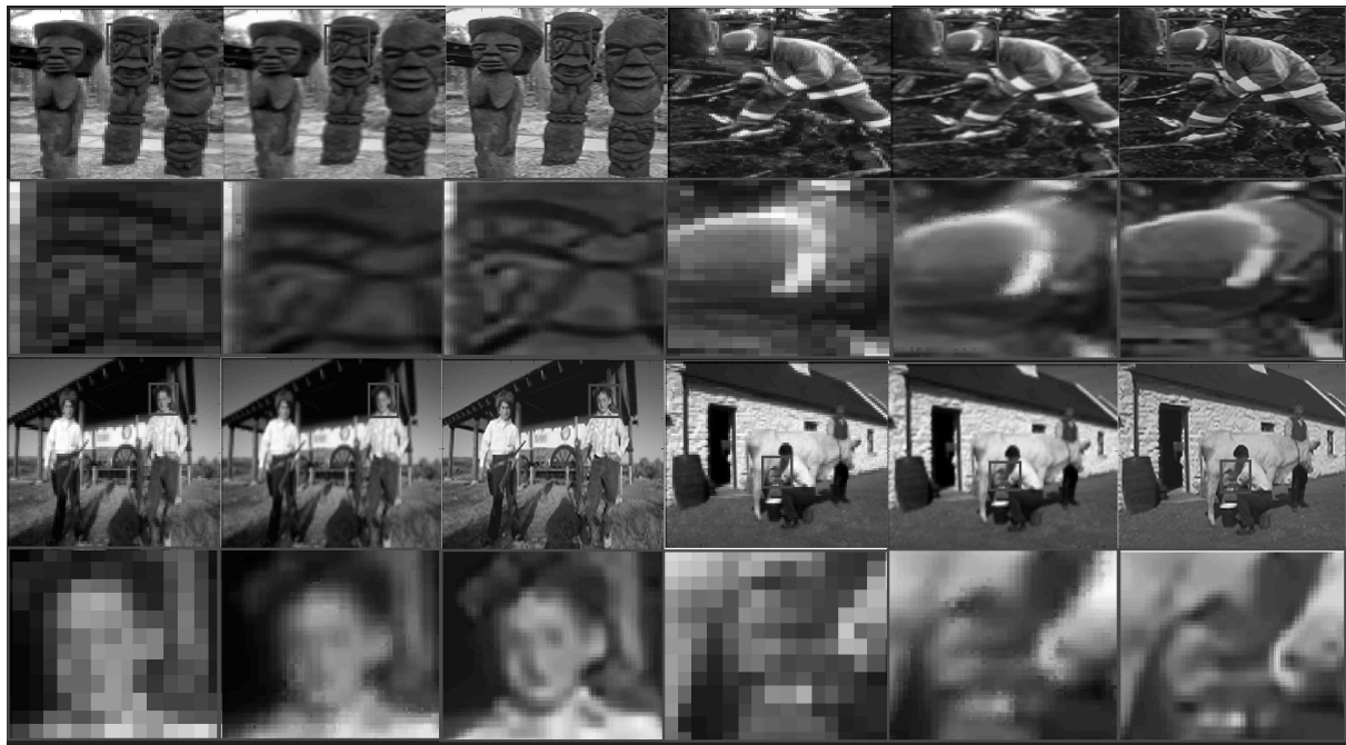
Figure 7. In the figure, left to right, the input image, the ART-ARG and the ART-ARG-Dictionary over figures 1)Idols, 42)Boys 56)Firefighter and 75)Farm of BSD100 database using factor q=4 . The H_r image is first blurred with a 7 \times 7 Gaussian kernel with standard deviation 1.6, and then down-sampled by a total scaling factor q in both horizontal and vertical directions. The PSNR/SSIM gains of our proposed method ART-AG-Dic over bicubic interpolation in each case are 1) 0.6dB/0.07 2) 1.8dB/0.06 3) -0.16dB/0.03 4) 1.5dB/0.07.
