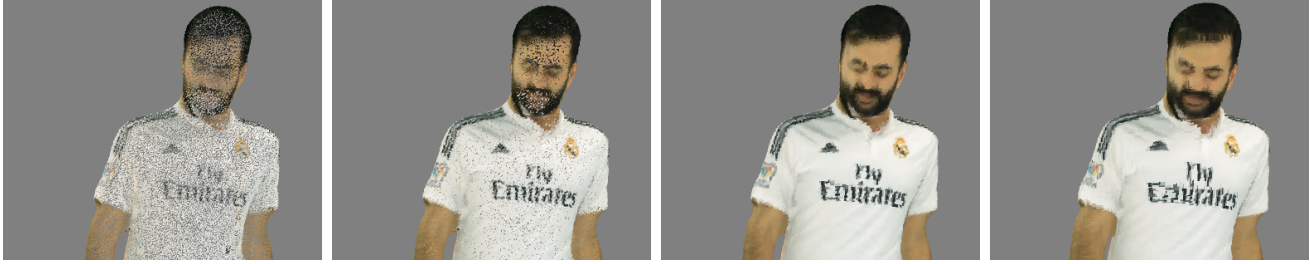
Figure 3. Four different sample rendered images showing the effect of point size on rendered images. Splat size increases from left to right. The holes are visible in the leftmost and centre-left images, and the rightmost image looks swollen, as the text on chest also changes shape. Thus, the splat size corresponding centre-right image was selected.
