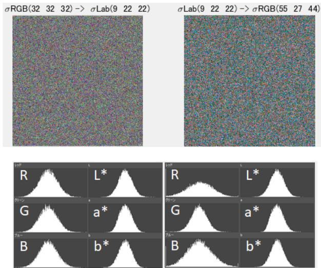
Figure 8: applying uncorrelated noise to an sRGB image results in different L\* a\* and b\* sigma levels (left). Applying those sigma levels to an Lab image as uncorrelated noise and converting them back to sRGB it leads to different sigma levels for the RGB channels (right).
