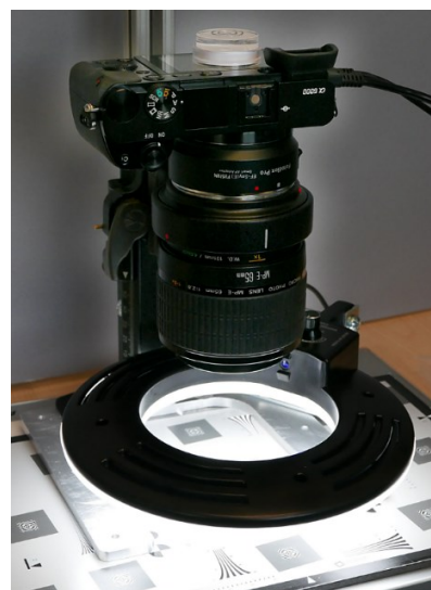
FIGURE 1. CHART MTF MEASUREMENT SETUP
