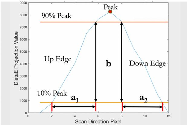
Figure 6: Calculation sharpness using the  $\Delta E$  projection of one streak.
