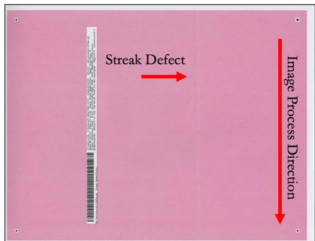
Figure 1: Test image with developer streak defect.
