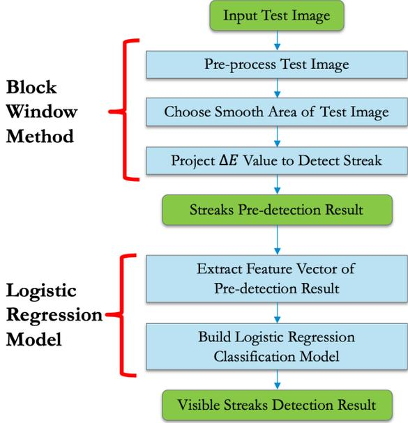
Figure 2: The overall pipeline of the streak detection method.
