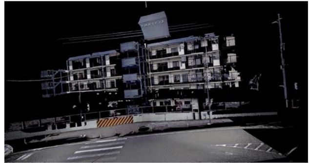
Figure 4. Generated image from the LiDAR point cloud.
