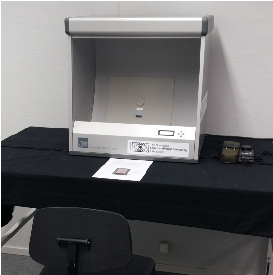
Figure 4. Experimental set-up in lit room: Viewing booth with a sample placed inside, held in place by a magnet, and a chair placed in front of the table for the observers to sit.
