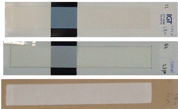
Figure 3. From top: White CT2846 substrate with a black strip and coated with white ink, clear Melinex coated with white ink and mounted onto white paper with a black strip, and kraft paper coated with white ink.
