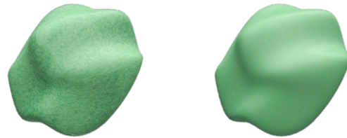
Figure 1. Comparison between a printed appearance (left)—highlighting its non-uniformities—and the computed ideal uniform (right).
