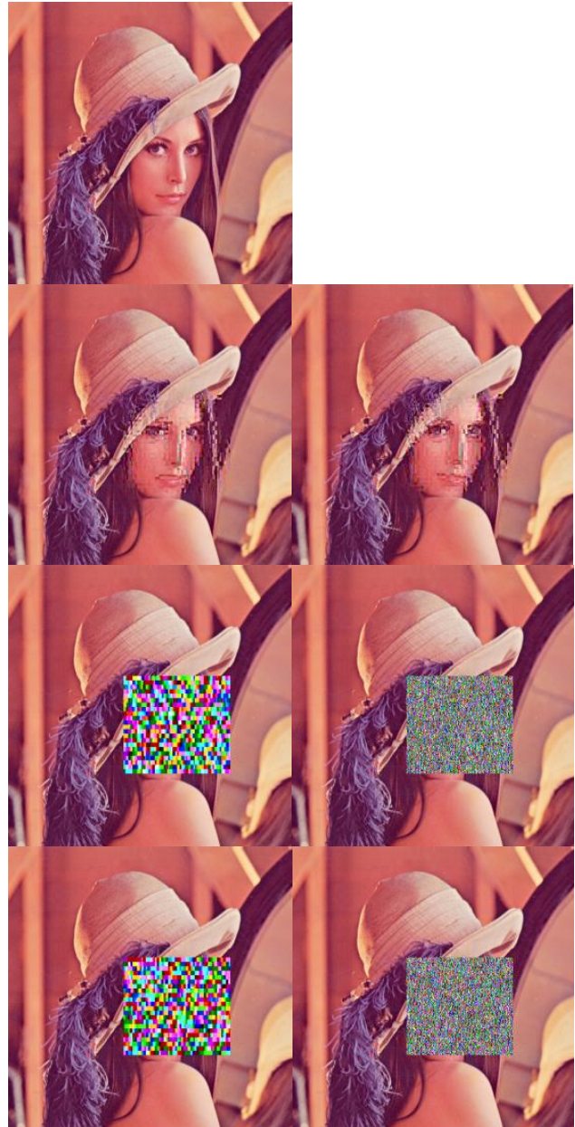
Figure 1. Visual impact. First line: Original. Second line: Coding-friendly encryption with 8 (left) and 64 (right) coefficients. Third line: Full encryption with 2 and 32 coefficients. Fourth line: Hybrid encryption with 2 and 32 coefficients.
