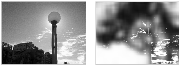
Figure 12. Falsely identified areas due to strong noise caused by high ISO during exposure.
