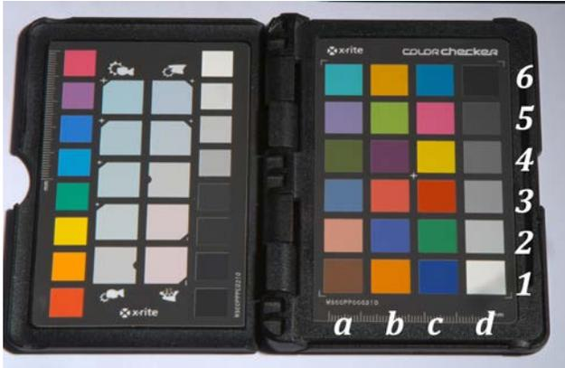
Figure 4. GretagMacbeth ColorChecker (pocket version) and identifiers used in the test
