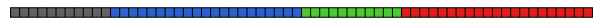
Figure 5. The default octant key design with 53 available bits. The red slots represent the amount of bits reserved for the X-coordinate, green represents Y and blue represents Z. The grey slots are unusable.
