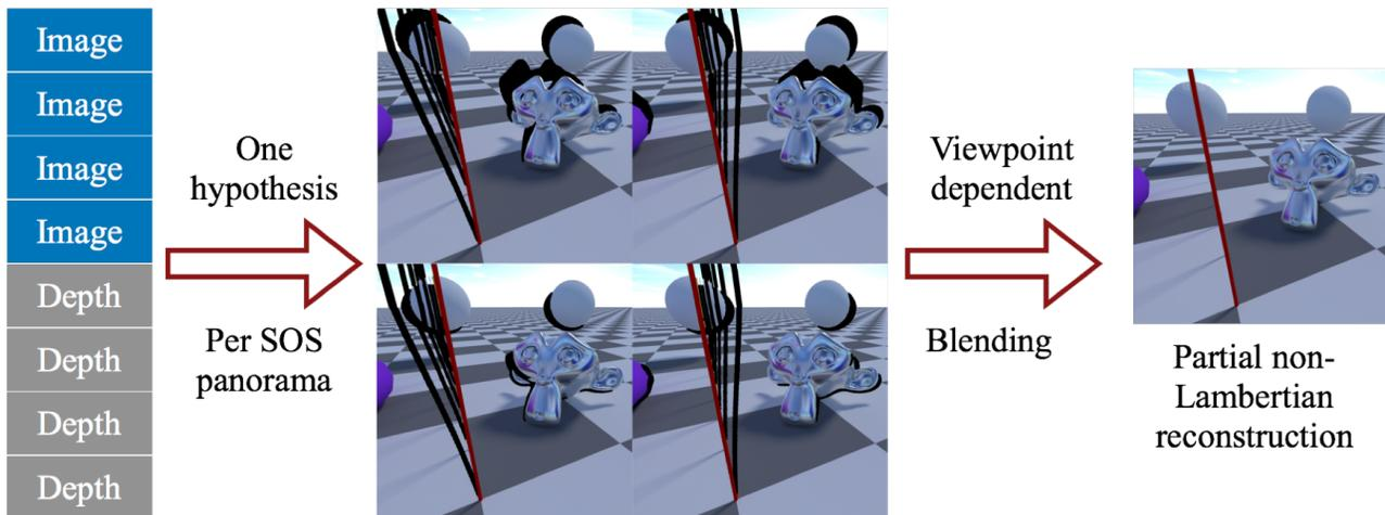
**Figure 8.** Hypothesis Merging: 4 SOS panoramas give rise to 4 hypotheses for the target viewpoint. The disocclusion holes appear in different directions around a foreground object in the different hypotheses, as shown. Thus, the holes get filled in the final view usually without inpainting.
