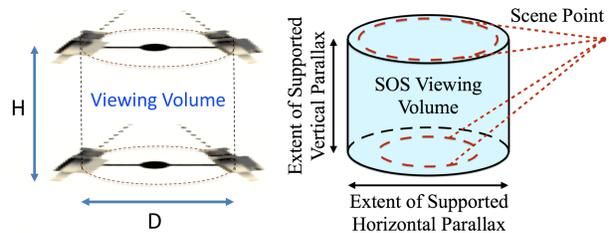
**Figure 5.** Left: A visualization of how SOS could be constructed from 4 cameras on a turn table. In practise, however, the representation would be typically constructed from a camera rig system. Right [8]: Each point in the scene gets recorded from 4 distinct viewpoints, as shown.
