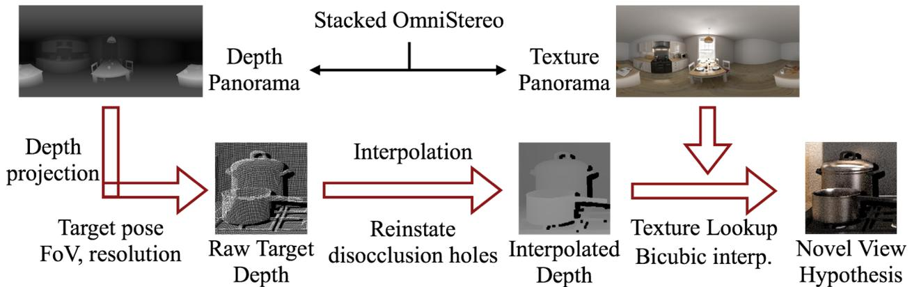
**Figure 6.** Hypothesis generation: Each SOS texture-plus-depth panorama is used to generate one hypothesis for target viewport. This is done using 3 steps as shown: forward depth projection, depth interpolation, and backward texture lookup. The 4 SOS panoramas generate 4 such hypotheses.
