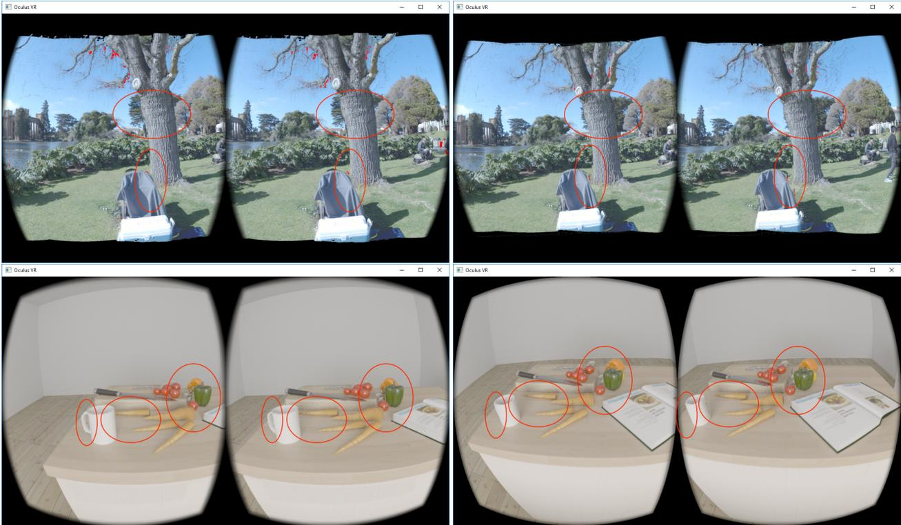
**Figure 10.** Motion parallax using the proposed system, rendered on a head-mounted display: Each row shows novel stereo views from two distinct viewpoints within the SOS viewing volume. The ellipses show the regions where the parallax is most noticeable. Top row: A natural scene captured using Facebook Surround 360. Bottom row: A photorealistic synthetic scene.
