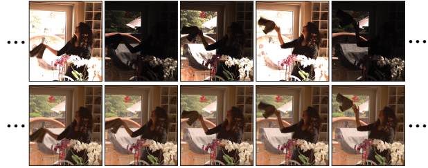
Figure 7. Stack-based acquisition for HDR video. The top row shows the captured frames with three alternating exposures. The bottom row shows the HDR video result reconstructed by the patch-based algorithm of Kalantari et al. [22].
