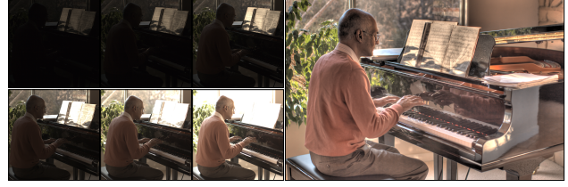
Figure 5. Deghosted HDR results from the patch-based optimization of Sen et al. [39] on the (cropped) input LDR images shown.
