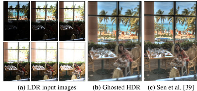
Figure 1. (a) Stack of differently exposed images of a scene. The limited dynamic range of the camera makes it unable to capture the interior and exterior simultaneously, even though it was perfectly visible to the naked eye. (b) High-dynamic range (HDR) image produced with the original merging algorithm of Debevec and Malik [6] that leverages well-exposed information from each image in the stack (see Eq. 1). Although the result contains well-exposed detail in all regions of the image, there are objectionable ghosting artifacts because of subject and camera motion while the stack was captured. (c) Result from the patch-based deghosting algorithm of Sen et al. [39]. This result captured the full range of illumination without the ghosting artifacts. All HDR results in this paper have been tonemapped for display.
