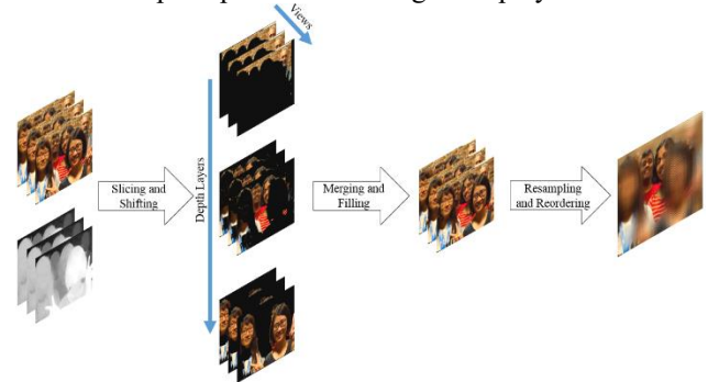
Figure 3. Flow diagram of the light field retargeting Block diagram of light field retargeting technique shown for 3 horizontal views and 3 disparity layers with central ZDP.
