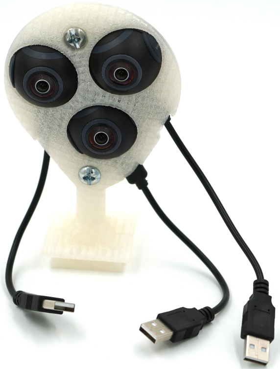
Figure 14. Kodama uses three cameras, six lenses, for 360° TDCI
