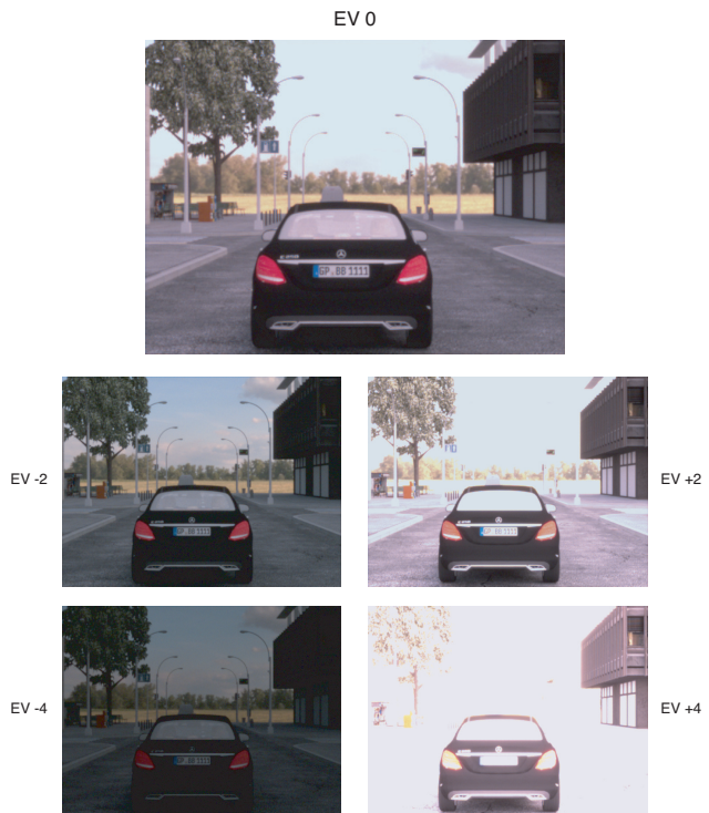
Figure 6: A simulated scene captured with the correct exposure value (top), under-exposed (left), or over-exposed (right). Such images, with different amounts of exposure value bias, were used for training and testing to explore network resilience to imperfections in the auto-exposure algorithm.
