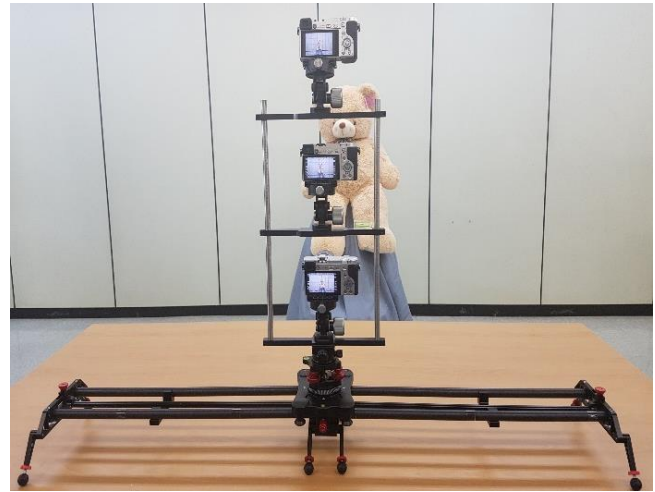
Figure 7. The proposed Full-parallax and high-quality multiview 3D image acquisition method using camera slider
