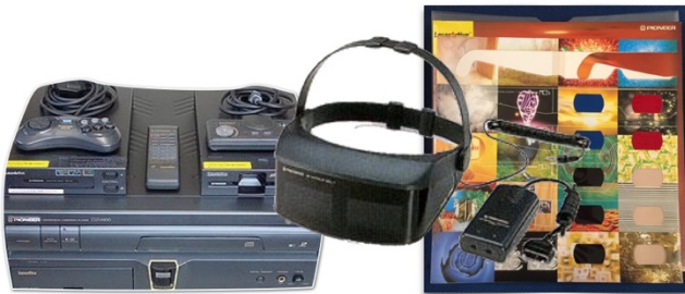
Fig 9. Pioneer LaserActive, Nintendo & NEC Extension PACS shown on top of the unit, Pioneer LaserActive Shutter Glasses, a tip-in sheet of perforated tear out Passive Glasses included with 3D Museum
