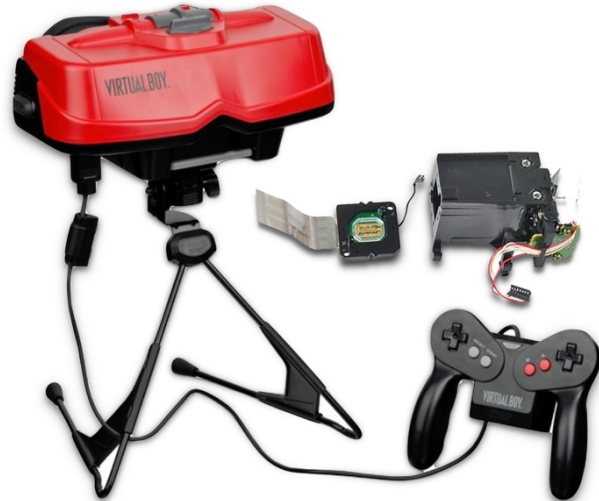
Fig 10. Virtual Boy Console and Controller, Shown with Internal Components for SLA and Mirror Array
