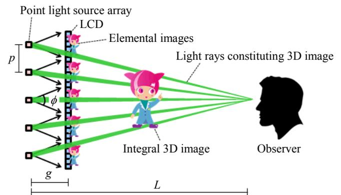
Figure 1. Principle of integral imaging system using point light source array.
