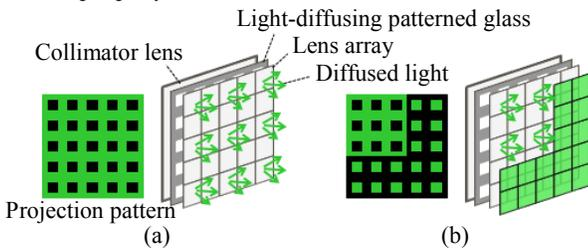
Figure 5. Examples of projection pattern to reproduce 2D image on: (a) entire display screen, (b) partial region of the display screen.
