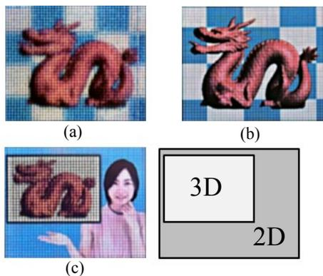
Figure 9. Reproduced images by 3D/2D switching display: (a) 3D image, (b) 2D image, (c) 3D and 2D images on partial regions.
