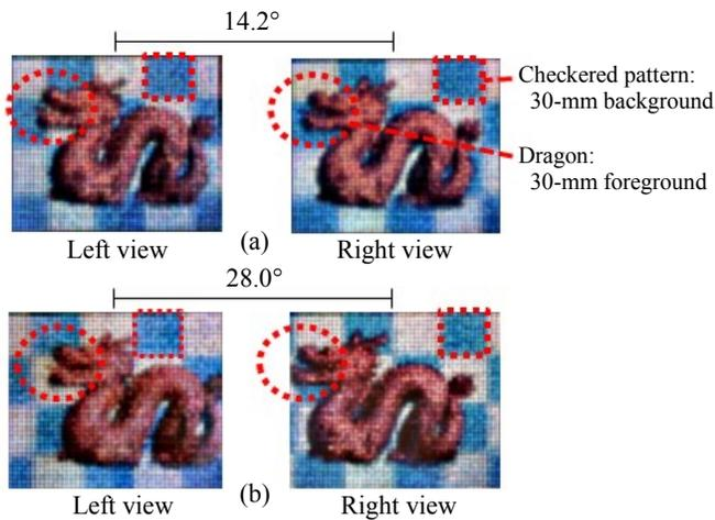
Figure 8. Viewing angle enhanced integral 3D image by time division display: (a) before enhancement, (b) after enhancement.
