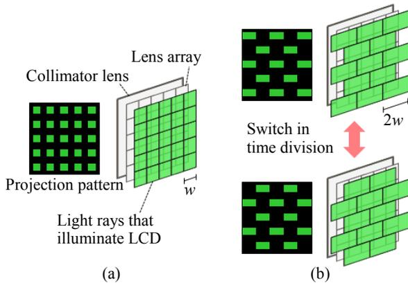
Figure 4. Examples of projection pattern to reproduce 3D image: (a) without time division, (b) with time division to enhance the horizontal viewing angle by twofold.
