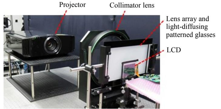
Figure 6. Prototype display system.
