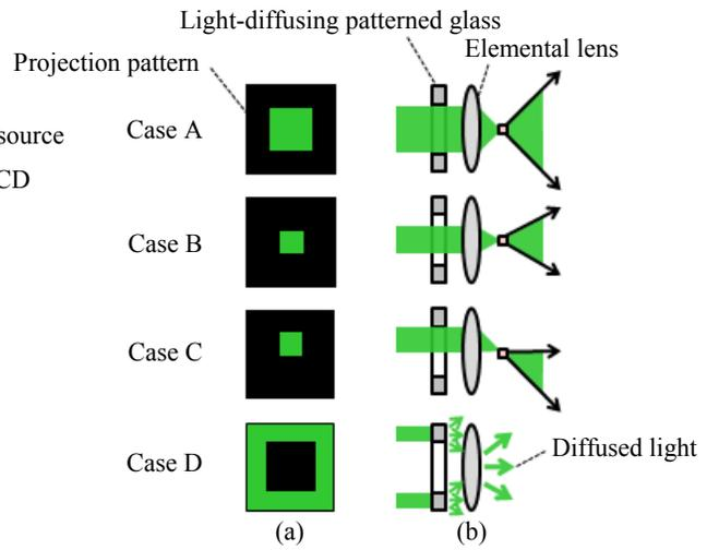
Figure 3. Example of projection pattern corresponding to elemental lens: (a) projection pattern, (b) path of light rays.
