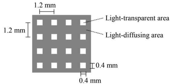
Figure 7. Structure of the light-diffusing patterned glass (partially enlarged).
