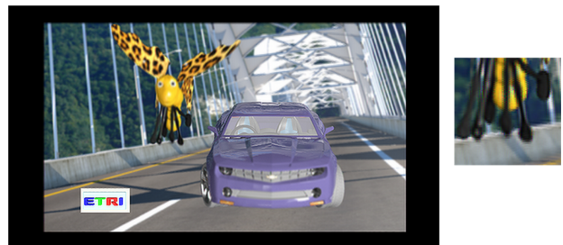
Figure 10. Eye view from multiplexed image which is obtained by nearest-neighbor interpolation from filtered DSLF.
