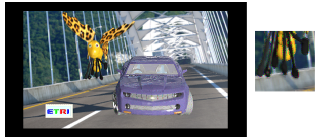
Figure 9. Eye view from multiplexed image which is obtained by nearest-neighbor interpolation from original reconstructed DSLF.
