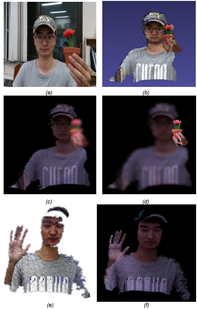
Figure 8. (a) Real 3D object of a person and (b) point cloud model 71221 points and 349 depth grids. Numerical reconstructed images with central positions located at (c) 200 mm and (d) 300 mm (e) point cloud model from a real sense 56876 points and 158 depth grids (f) Full-color reconstructed images with central positions located at 200mm.
