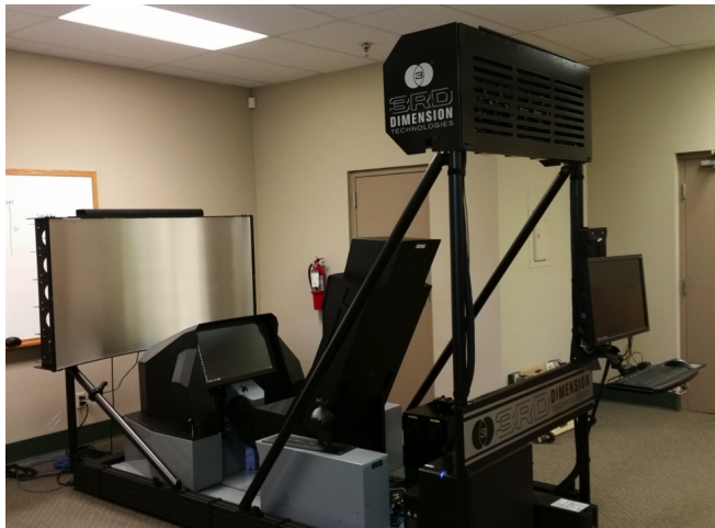
Figure 4. Image of Flight Simulator with Integrated TDT High Resolution FoLD System
