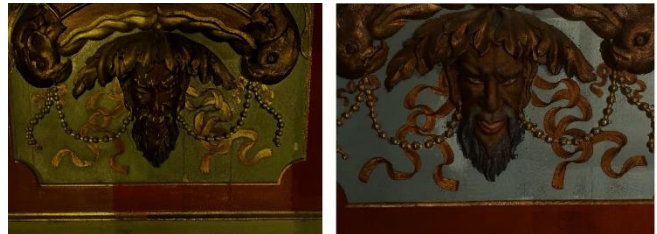
Figure 2. Visual comparison between two registered point clouds from 2011 (left) and from 2015 (right)
