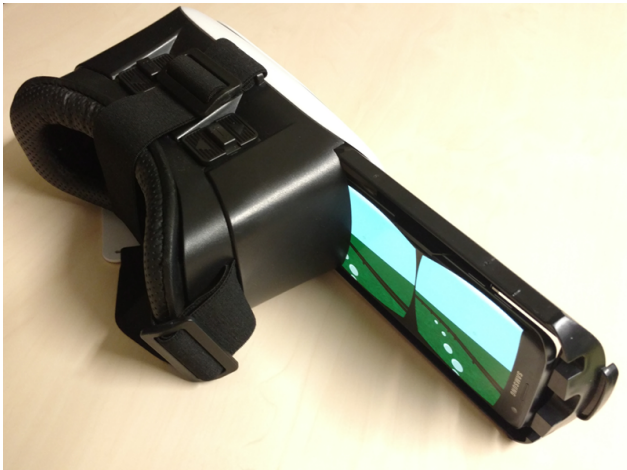
Figure 12. Visensor/VR: Running on a smartphone inside the VR Box in side-by-side view
