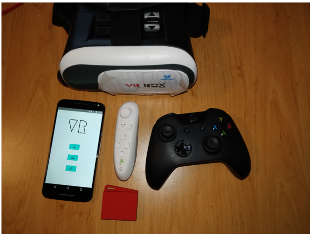
Figure 1. Hardware used in the projects: VR Box (top), smartphone (Samsung Galaxy S6, left), Texas Instruments SensorTag CC2650 (bottom). SensorTagVR: VR Sensorpark (center), Visensor/VR: XBOX controller (right).
