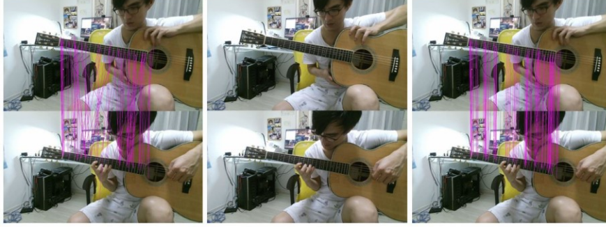
Figure 2a: Left: SIFT Matching Result; Middle: Traditional RANSAC (cannot calculate Homography due to too many outliers); Right: Filtered Matching Result Based on Our Modified RANSAC
