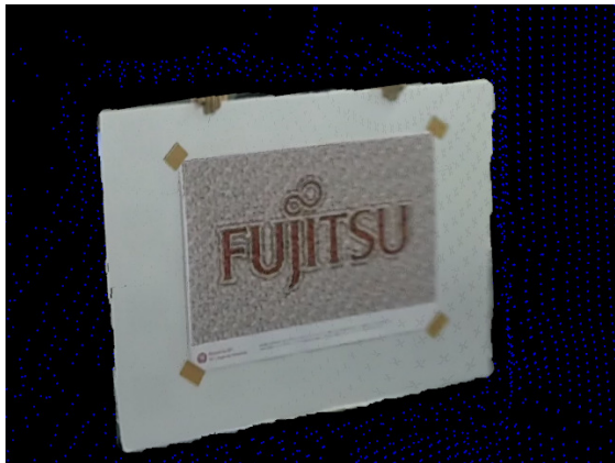
Figure 11. Up-sampled synchronized 3D point cloud with planarity constraint
