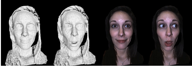
Figure 6. Compressing encoded 3D data with the H.264 video codec at very lossy (CRF of 25) qualities achieving a 16,279:1 compression ratio.
