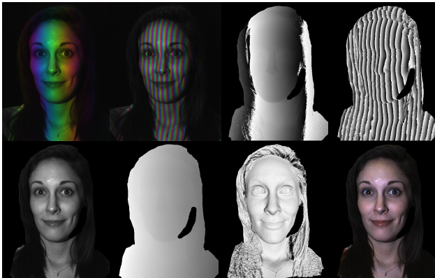
Figure 2. Example of reconstructing 3D geometry and color texture from the Acquisition Module. Top row left to right: low frequency fringe patterns, high-frequency fringe patterns, low frequency wrapped phase \phi^l , high-frequency wrapped phase \phi^h ; bottom row left to right: b/w texture I_t^g , unwrapped phase \Phi , 3D geometry, color texture after demosaicing I_t^c .
