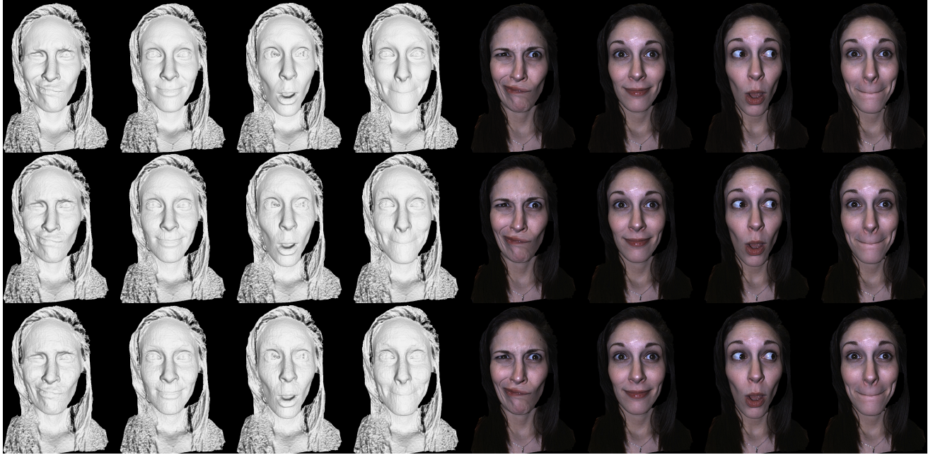
Figure 4. Compressing encoded 3D data with the H.264 video codec at different qualities. First row: four frames decoded from the video stored with lossless H.264 (compression ratio 129:1); second row: four frames decoded from H.264 video using 4:2:0 subsampling and a constant rate factor of 6 (compression ratio 551:1); and third row: the corresponding frames using the same encoding instead with a constant rate factor of 12 (compression ratio 1,602:1).
