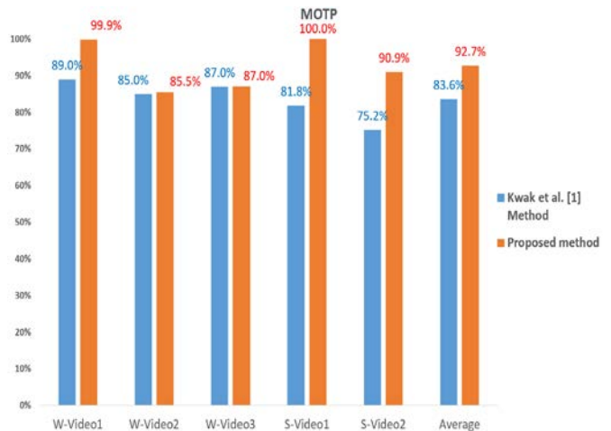
Fig. 3. MOTP performance comparison of the two methods about five thermal video sequences
