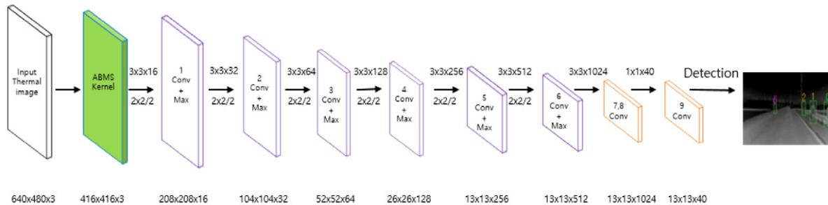
**Figure 2.** Illustration of tiny YOLOv2 adopting a handcrafted ABMS kernel. Tiny YOLOv2 consists of nine convolutional layers and six max pooling layers followed by two fully connected layers. In our system, ABMS is applied as the initial handcrafted kernel. The input image is first applied to the ABMS kernel, and a saliency map is transferred to the YOLO network.
