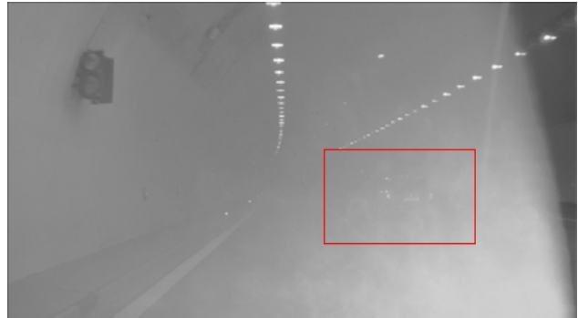
Figure 1: A scene while entering a tunnel with veiling glare on the windscreen due to dust particles. A human observer may still resolve the car due to a good contrast detection ability of the human eye
