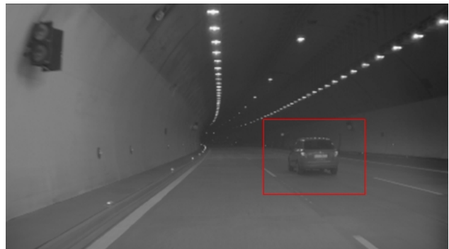
Figure 2: The same scene as in fig. 1 but now the veiling glare has disappeared. Inside the video-stream an object has suddenly appeared.
