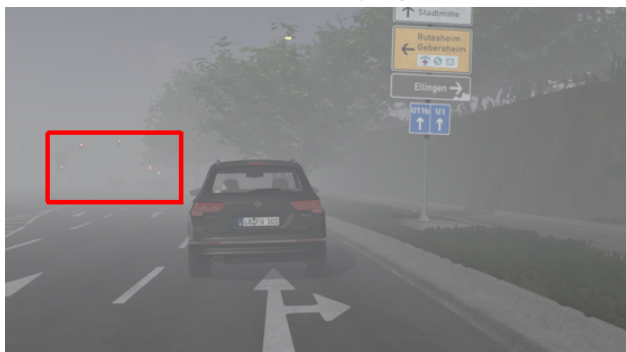
Figure 5: The reference scene with strong fog. The objects in the red box are not detectable any more and even the contrast loss of nearby objects decreased to a level that texture extraction may fail.
