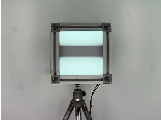
Figure 11. Image captured during 60Hz test. A dark band is visible in the middle of the light. The band is a rolling shutter effect
