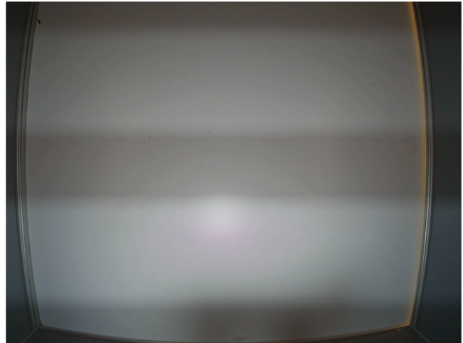
Figure 4. Example of banding artifact. This image was captured with a rolling shutter sensor. In this example, the scene is illuminated by a diffuse LED light source, driven by a 75Hz, 10% duty cycle signal
