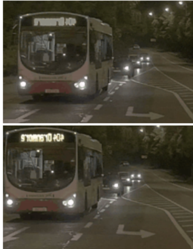
Figure 7. Example of HDR PWM flicker in lowlight scene. Two consecutive frames from a video sequence are shown. The sign is driven by a PWM signal. In frame N (top), the bus sign is captured only by the long exposure and missed by the short exposure. The combined output is a mid-grey artifact with no detail. In frame N+1 (bottom), the bus sign is captured by the short exposure, and is therefore reproduced correctly in the combined HDR output image
