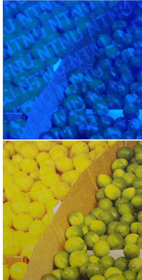
Figure 8. Printed sample under UV (top) and D50 (bottom). The object detail is coarse enough to not interfere with the watermark.
