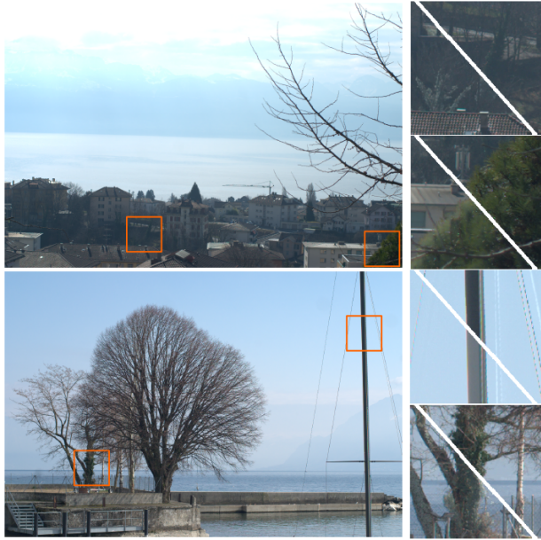
Figure 4. Original hazy images (left) and crops of results obtained after dehazing (right) using our algorithm (top) and the algorithm proposed by Schaul et al. [6]. Artificially bright regions resulting from high material reflectance properties are corrected using our algorithm.
