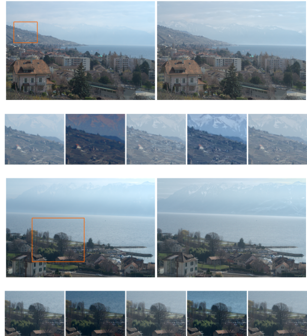
Figure 5. Original and dehazed images using our approach (full images) and comparison with state-of-the-art results (zooms). From left to right are depicted: original image, He et al. [22], Schaul [6], Feng et al. [28] and our result. Our method gives state-of-the-art dehazing results while conserving the colors of haze-free regions, thus yielding photorealistic dehazing.
