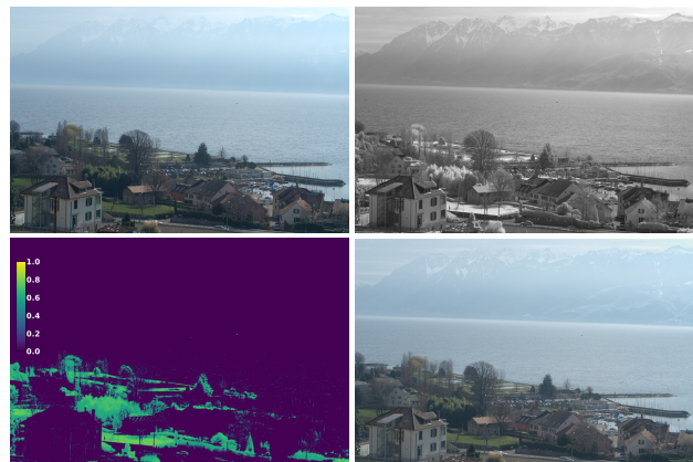
Figure 1. Image dehazing results obtained using the proposed algorithm. From top left to bottom right are shown the hazy input image, NIR image, inconsistency mask, and the dehazed image. Note how the details of the NIR image are merged with the RGB image without changing the color of non-hazy regions such as the port in the bottom of the image.
