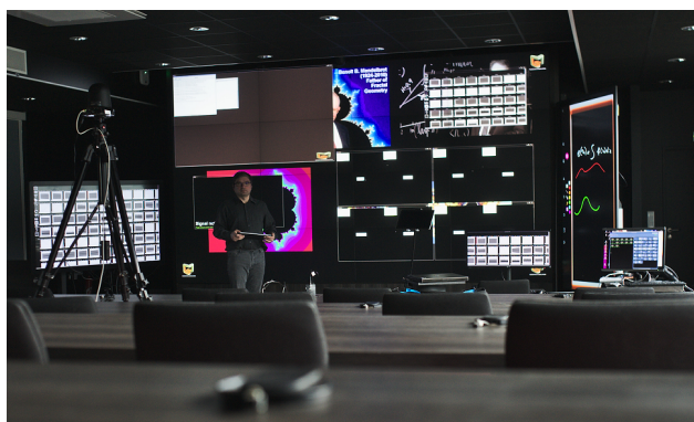
Figure 1. Overview of the MANDELBROT platform: from left to right: the tactile table, a tripod for a camera, the display wall and a vertical touch screen used as a black board.
