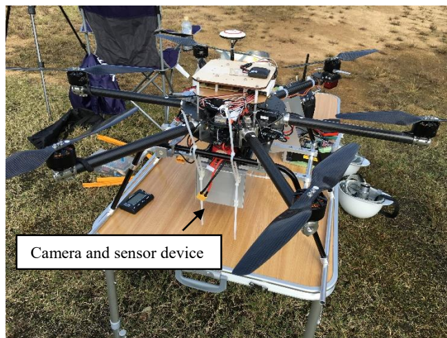
Figure 8. UAV with 6 rotors used in the experiment. We attached the camera and sensor device so that it faces downward at the center of the fuselage.
