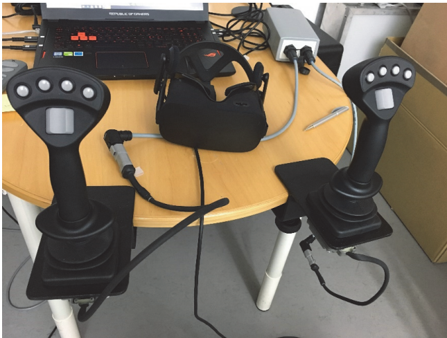
Figure 2: The two joysticks for operating the crane in the VR simulator and the HMD of the brand Oculus Rift
