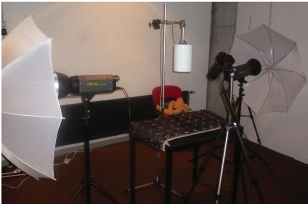
**Figure 2.** Picture of the experimental set-up. The collimated light was positioned at a fixed distance from the centre of the table ( $d = 0.50$  m). The angle of incidence was varied from directly above (0 deg) to 75 deg to the right.
