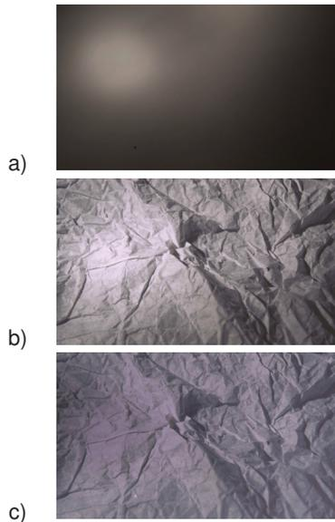
**Figure 3.** a) Luminance gradient on matte white photography paper under collimated lighting at 0 deg angle of incidence. b) Image before rescaling. c) Image after rescaling.
