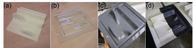
Figure 1. Stimuli construction. (a) Surfaces were first carved from polymer foam using a CNC machine. (b) These molds were later used in a vacuum-forming machine to create the plastic surfaces. Plastic surfaces were spray-painted in either a single color (c) or with two colors side by side (d). Figure reproduced from [22].
