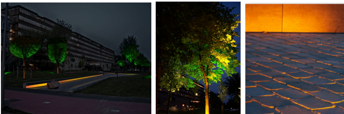
Figure 4 Left: a computer rendering of a part of a lighting plan. Middle and right: two photographs made during an evening workshop, in which the intended visual effects were tested. Middle: a photograph in which the colors of the canopy show two different colors – tree colors appear very sensitive to the exact lighting spectrum and it is advised to always test such effects on the spot. At right a photograph of a test of the lighting of the curb, for which the direction and beam shape are important determinants of the effects. In the rendering these could be fine-tuned quite easily – but due to the simplified material models the effects of the grazing lighting on the cobble stones could not. (and actually resulted in a very nice texture)
