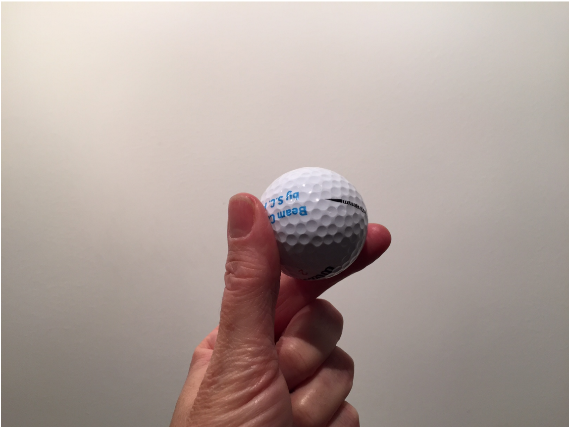
Figure A1. Light in front of a wall, with a “light probe” –an object to visualize the light qualities- in the light. Here we use a golf ball for which it was proven that the intensity, direction and diffuseness of the light can be judged well from the shading and 3D texture gradients [Xia et al., 2014].
