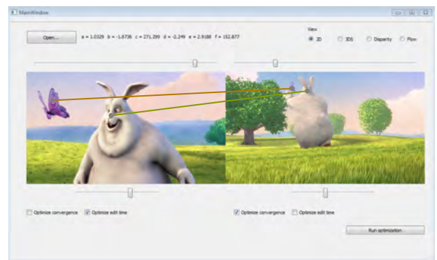
Figure 7: Optimization of film editing operations to best match the human depth adaptation abilities based on the vergence response time model. The colors of the lines connecting points of interest before and after the cut visualize the corresponding vergence adaptation times. Pictures from Big Buck Bunny by Blender Foundation.
