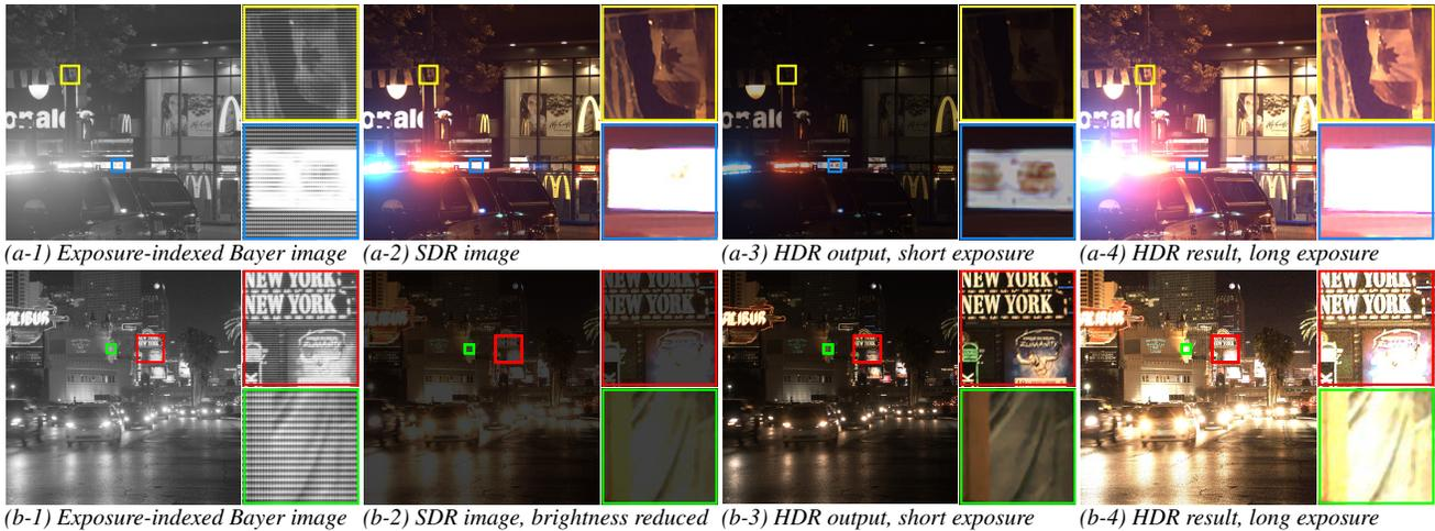
**Figure 7:** Results. The grey image on the left column shows the input exposure-multiplexed Bayer image. For our HDR reconstruction, both a short and a long simulated exposure is shown, for the demonstration of the quality of our reconstruction. Details are shown in the blown up insets.
