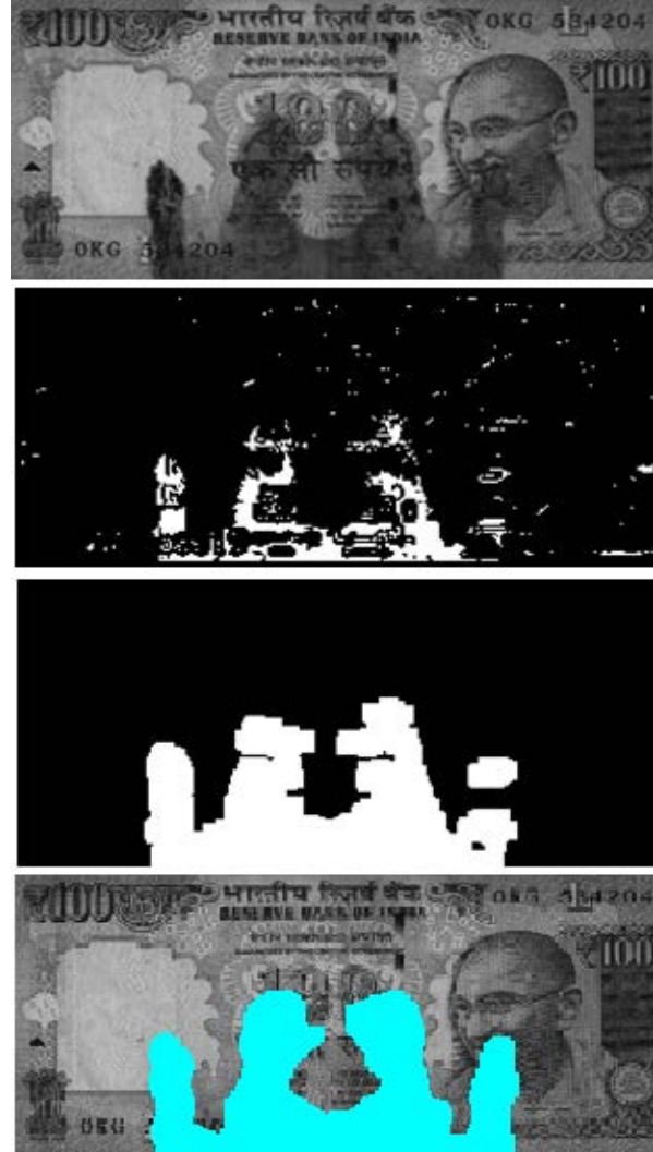
Figure 7. (a) target image, (b) threshold map, (c) decision map, (d) ground truth image of the 100 rupees image.
