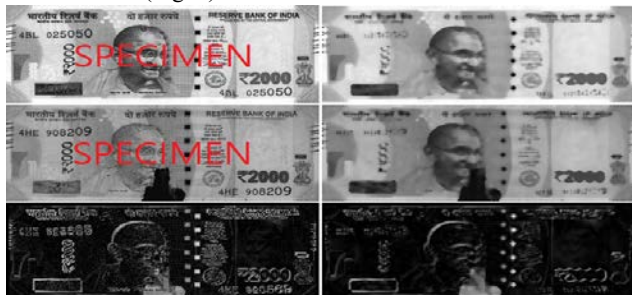
Figure 1. (a) reference, (b) median filtered reference, (c) target, (d) median filtered target, (e) difference image, (f) median filtered difference image.
