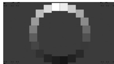
Figure 3. Test target used for noise measurement according to ISO 15739:2013 (TE264)- the chart consists of 20 uniform gray patches.
